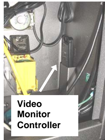
Figure 13 Video monitor remote controller in its storage position in the middle tower section.
