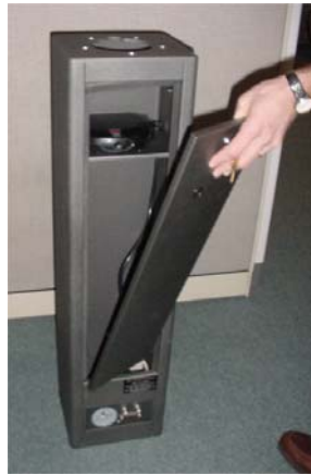
Figure 3 Removing the covers to help with lifting and handling the tower sections.
