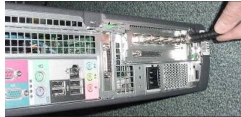
Figure 10 Connecting video cable to frame grabber board on Lane PC.
