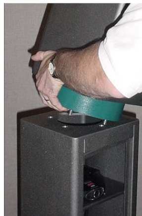
Figure 6 Supporting the spacer ring and aligning screws to set upper/middle section onto lower section.
