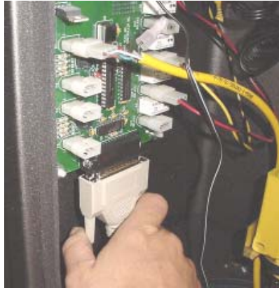
Figure 8 Connecting the DB-25 cable to the tower controller (printed circuit) board.
