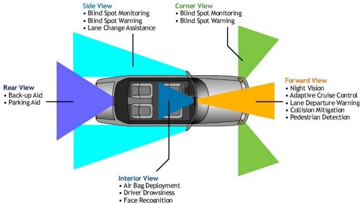
Figure 3 Applications of cameras in automotive safety
